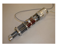
A SEA (Series Elastic Actuator) to be used as a robotic leg, realized from the laboratory company Robot Factory.
